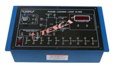
Experimental Training Board has been designed specifically for the study of Phase Locked Loop (PLL) IC 565. This training board covers most of the important parameters, characteristics and applications on Phase-locked Loop (PLL) IC 565.
