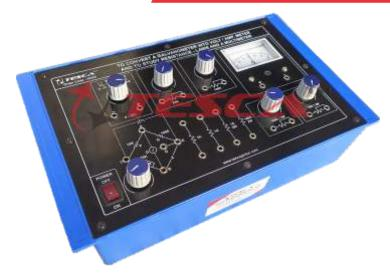
**36200** Experimental Training Board has been designed specifically for a detailed practical study of conversion of a Galvanometer into a Volt / Amp meter and study of the laws of Resistances. The unit has an added feature that you can also learn to use a Multimeter.
