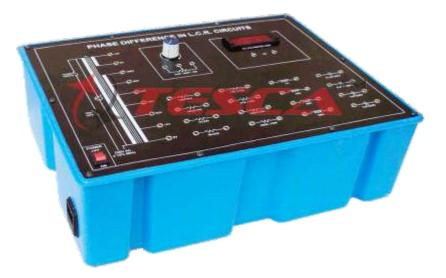
36201 Experimental Training Board has been designed specifically for the complete study of the phase difference in L.C.R. circuits. A selection of L,C and R values have been provided and phase difference in various combinations of L-C, L-R, C-R and L-C-R circuits can be studied in depth. The board is absolutely self contained and requires no other apparatus.
