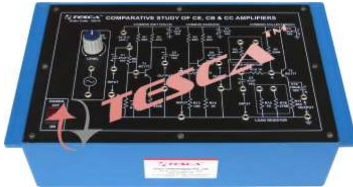
Experimental Training Board has been designed specifically for the Comparative study of Common Emitter (CE), Common Base (CB) and Common Collector (CC) Transistor Amplifiers. These practical transistor amplifier configurations are evaluated in respect of their main parameters and results are compared with theoretical calculations.
