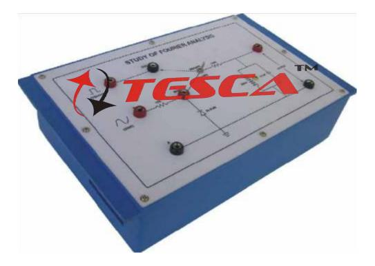
Experimental Training Board has been designed specifically for the study of Fourier Analysis. In electronics, we deal with signals which are not simple Sine Waves. They are composed of a number of Frequencies and their description is quite complex. However, any complex signal may be represented as a sum of simple Sine or Cosine waves. The mathematical tool that helps us in this type of analysis is called the Fourier theorem.
