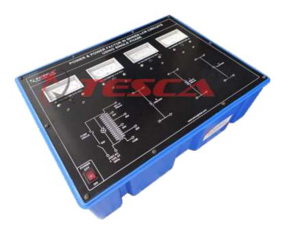
Experimental Training Board has been designed specifically to determine the Power and Power Factor in Series RLC circuit using Single Phase A.C. Supply. The board is absolutely self contained and requires no other apparatus.
