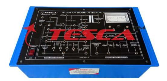
Experimental Training Board has been designed specifically for the study of Amplitude Modulation and demodulation with basic Diode detector. The Training Board is helpful for the study of improved Diode Detector and detection of efficiency of a diode in Amplitude Modulation and Demodulation.
