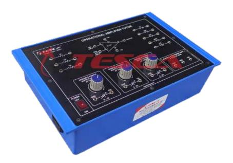
Experimental Training Board has been designed specifically for the study of basic Applications of Operational Amplifier (OP-AMP) using IC-741.
