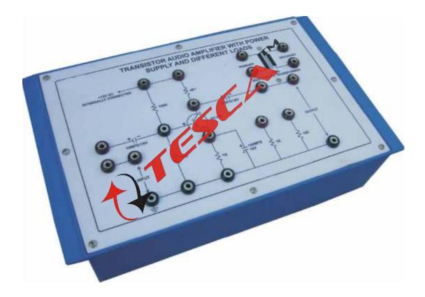
Experimental Training Board has been designed specifically for the study of single stage Transistor Audio Amplifier with three different loads.
