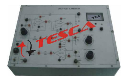
Experimental Training Board has been designed specifically for the study of Active Limiter using OP-AMPICs 741. This Training Board gives a better understanding of the principles of limiting of input voltage at output with specified limits of +ve & -ve voltages. The board is absolutely self contained and requires no other apparatus.
