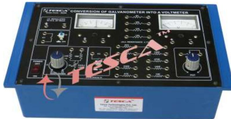
Training Board has been designed specifically for study of Conversion of a Galvanometer into a Voltmeter. The board is absolutely self contained and requires no other apparatus.
