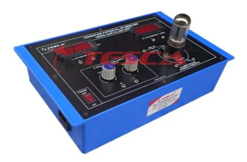
Experimental Training Board has been designed specifically to find the ionisation potential of mercury using gas filled diode. The board is absolutely self contained and requires no other apparatus.
