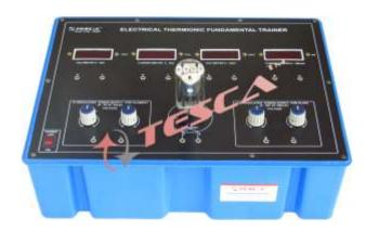
Experimental Training Board has been designed specifically for to determine the therminoic work function of tungsten using a directly heated valve and Verification of Richardson's Equation of thermionic emission. The board is absolutely self contained and requires no other apparatus.
