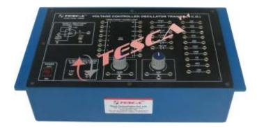
Experimental training board has been designed specifically for the study of Voltage Controlled Oscillator (V.C.O.)
