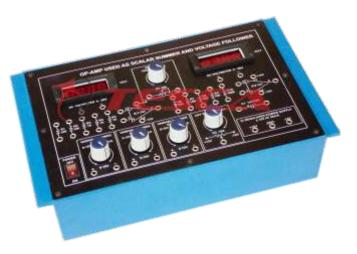
36303 Experimental Training Board has been designed specifically for the study of Scaling, Summer and Voltage follower using OP-AMP ICs 741.
