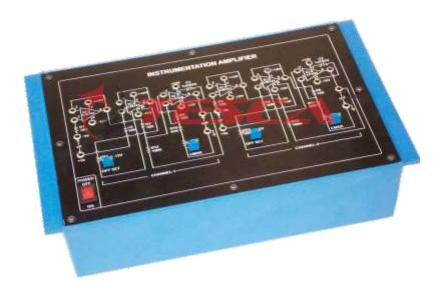
**36306** Instrumentation Amplifier trainer has been designed specifically for the study of differential - input of Instrumentation Amplifier in a closed loop and it differs fundamentally from the standard OP-AMP.
