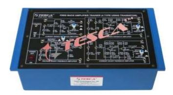
Experimental Training Board has been designed specifically for study current series, current shunt, voltage series and voltage shunt Feed Back Amplifier using Transistors.
