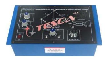
The experimental set up has been designed specially for the study of To Measure the Value of Unknown Self Inductance.
