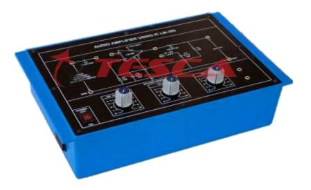
36323 Experimental Training Board has been designed specifically for the study of Audio Amplifier using LM-380.
