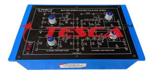
39329 Experimental Training Board has been designed specifically to study. First & Second order of Low Pass Butterworth Filter for a higher cut off frequency of 1 KHz with a pass band gain of 2 & First & Second Order High Butter worth filter for Lower cut off frequency of 1 KHz with a pass band gain of 2. Practical experience on this board carries great educative value for Science and Engineering Students.
