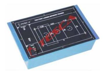
Two Port Ladder Trainer 36336 is a useful trainer to illustrate the importance of Transfer Function of two port ladder network. It is the general configuration of a ladder network in which series arm is represented as Impedance arm and Shunt arm is represented as Admittance arm.
