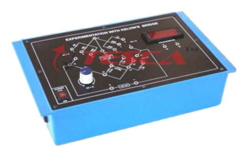
36362 (Experimentation with Kelvin's Bridge) is useful training product for measuring very small values of resistance, Kelvin's double bridge or Kelvin's bridge (as it is commonly known as) is a variation of wheatstone bridge and is based on the same principal. By setting the null point we can evaluate the unknown resistance.
