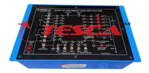
Computer Logic Training Board has been designed specifically for the study of Arithmetic & Logic function by using 74181 chip. The board is absolutely self contained and requires no other apparatus.
