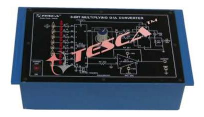
To Study 8-Bit Multiplying Digital to Analog Converter with 8-Bit Input Digital Signals and Analog output signal representing the product of Inputs and Reference source.
