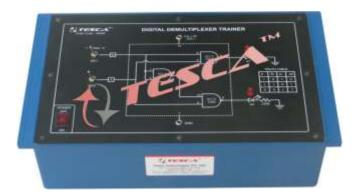
Computer Logic Training Board has been designed specifically to familiarise the operation of a demultiplexer circuits. In digital system the technique of multiplexer and demultiplexers are frequently used to reduce the system cost and to improve the reliability. The unit provides the understanding of two output demultiplexers. This concept can be extended to make the demultiplexers for more complex circuits. The unit is absolutely self contained and requires no other apparatus.
