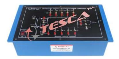
Computer Logic Training Board has been designed specifically for the study of 4-bit binary UP/DOWN counter. This Training Board gives a better understanding of counter using 4-bit presetable inputs, one master reset and parallel load with 4-bit BCD output. The board is absolutely self contained and requires no other apparatus.
