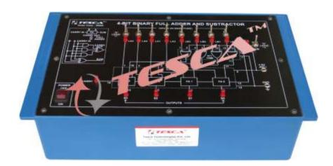
Computer Logic Training Board has been designed specifically for the study of phenomena of addition and subtraction of 4-bit binary numbers using 4-bit arithmetic and complementary techniques. This Training Board uses controlled inverter and full adders to carry out the operations of addition and subtraction. The board is absolutely self contained and requires no other apparatus. Practical experience on this board carries great educative value for Science and Engineering Students.
