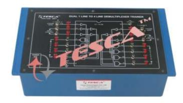
Computer Logic Training Board has been designed specifically for the study of Dual 1 Line to 4 Line Demultiplexer. The Training board gives a understanding of the phenomena of demultiplexing with DUAL one input (STROBE DATA) demultiplexed to four outputs using two control inputs (Address).
