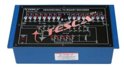
Computer Logic Training Board has been designed specifically for the study of Hexadecimal to Binary Encoder. The training board gives a understanding of the phenomena which encodes 16 data lines to 4 lines binary encoder. The board is absolutely self contained and requires no other apparatus.
