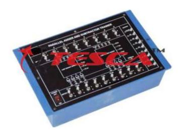
38697 Parallel Adder and Subtract or Trainer is a ready to use digital electronics experiment trainer. This product, has been designed specifically for the students to understand the concept of parallel binary addition and subtraction methods for-4- bit and 8 bit binary numbers.
