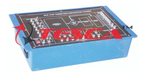
**38698** BCD Adder and Subtract or Trainer is a compact, ready to use digital electronics experiment board. This product has been designed specifically for the students to study and understand the concept of BCD addition and subtraction processes.
