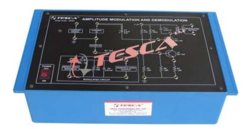
Experimental Training Board has been designed specifically for the study of Amplitude Modulation and Demodulation. This training board is based on latest solid state circuits for generating modulating signal, Amplitude Modulation and Demodulation.
