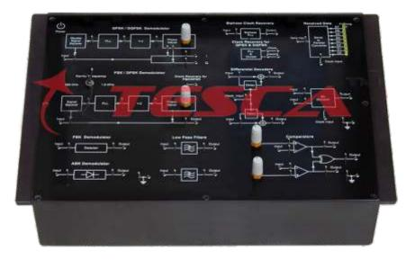
Carrier Demodulation & Data Reformatting Receiver 40533 is complete digital communication platform which efficiently explains all communication processing steps involved in reception of Digital signals. Various digital demodulation techniques viz. ASK, FSK, PSK, DPSK, QPSK etc. can be implemented using 40533.
