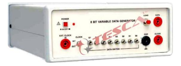
It can be used along with as a data input generator and also can be used independently as a 8-bit variable TTL data generator. It has a facility to fed external clock (TTL) upto 1 MHz which will be available at the Clock Out socket on the front panel. Otherwise it operates on internal 240 KHz clock.
