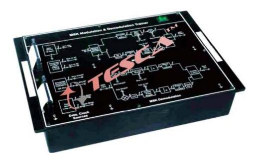
MSK Modulation / Demodulation Trainer is designed to assist students to understand the basic working principal of Minimum Shift keying technique. As the name suggests, MSK results in a modulation scheme which has smooth phase variations in contrast to other phase modulation schemes where the modulated signal contains abrupt phase changes. The immediate advantage of such a scheme is the reduction in modulated signal bandwidth. MSK Modulation / Demodulation comprises of following major blocks:
