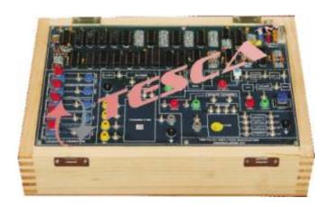
Order Code-40612 is a Digital Communication Trainer System to under stand various digital Modulation and Demodulation Techniques. Various functional block diagrams are provided on-board for Teaching/Training. This Kits provides with various Test Points to visualize the signals on Oscilloscopes.
