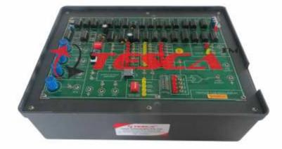
**Order Code-40613** is a Digital Communication Trainer System to under stand various digital Modulation and Demodulation Techniques. Various functional block diagrams are provided on-board for Teaching/Training. This Kits provides with various Test Points to visualize the signals on Oscilloscopes.
