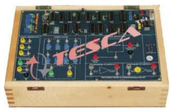
**Order Code- 40616** is a Digital Communication Trainer System to under stand various digital Modulation and Demodulation Techniques. Various functional block diagrams are provided on-board for Teaching/Training. This Kits provides with various Test Points to visualize the signals on Oscilloscopes.
