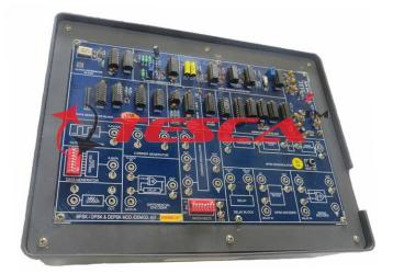
**Order Code-40619** is an Advance Digital Communication Trainer System that helps one under stand various Digital Modulation and Demodulation Techniques. Various functional block diagrams are provided on-board as an aid for Teaching/Training. These Kits are provided with various Test Points to visualize the signals on Oscilloscopes.
