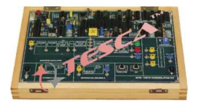
**Order Code-40621** is an Advance Digital Communication Trainer System that helps one under stand various Digital Modulation and Demodulation Techniques. Various functional block diagrams are provided on-board as an aid for Teaching/Training. These Kits are provided with various Test Points to visualize the signals on Oscilloscopes.
