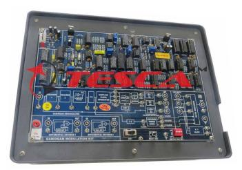
**Order Code-40624** is an Advance Digital Communication Trainer System that helps one under stand various Digital Modulation and Demodulation Techniques. Various functional block diagrams are provided on-board as an aid for Teaching/Training. These Kits are provided with various Test Points to visualize the signals on Oscilloscopes.
