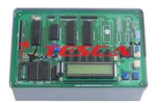
**43204** is a single board Microprocessor Trainer Kit based on 8085 Microprocessor, which is widely used to train engineers to develop software/hardware for any industrial process & control. This Kit consists of power-full Monitor EPROM, RAM, I/O Lines, Timer/Counter, Serial, 20x2 LCD Display and Keyboard for Man to Machine Interface.
