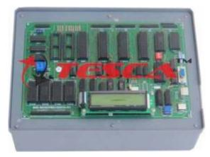
**43212** is a single board Microprocessor Trainer Kit based on 16 bit 8086 Microprocessor, which is widely used to train engineers to develop software/hardware for any industrial process & control. This Kit consists of power-full Monitor EPROM, RAM, I/O Lines, Timer/Counter, Serial, LCD Display and Keyboard for Man to Machine Interface.
