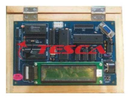
43213 is a single board Microcontroller Trainer Kit based on 8 bit 8051 Microcontroller, which is widely used to train engineers to develop on software/hardware for any industrial process & control. Kit has power-full Monitor EPROM, RAM, I/O Lines, Timer/Counter, Serial, LCD Display, Keyboard for Man to Machine Interface.
