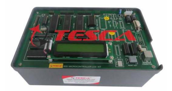
**43215** is a single board Microcontroller Trainer Kit based on 8 bit 8051 Microcontroller, which is widely used to train engineers to develop on software/hardware for any industrial process & control. Kit has power-full Monitor EPROM, RAM, I/O Lines, Timer/Counter, Serial, LCD Display, Keyboard for Man to Machine Interface.
