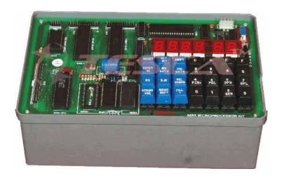
43219 is a single board Microprocessor Trainer Kit based on 8085 Microprocessor, which is widely used to train engineers to develop software/ hardware for any industrial process & control. This Kit consists of power-full Monitor EPROM, RAM, I/O Lines, Timer/Counter, Serial, Seven Segment Display and Keyboard for Man to Machine Interface.
