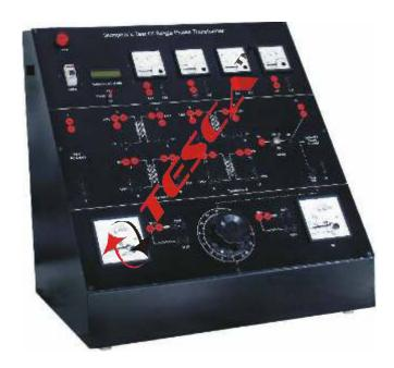
Sumpner's Test of Two Single Phase Transformers is a very exclusive and important product designed for students of Electrical Engineering to explain the basic concepts of Sumpner's test. With this trainer, students can learn about the significance of conducting the heat run test with two single phase transformers and correspondingly can determine the efficiency and voltage regulation Additionally one can also learn the phenomenon of polarity.
