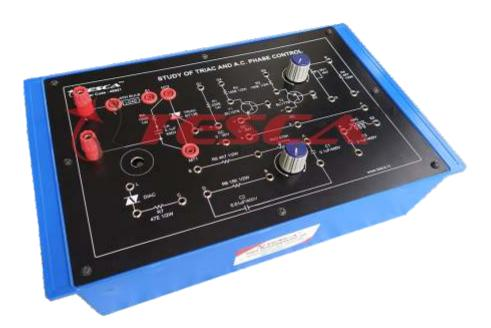
Power Electronic Training Board has been designed specifically to study the characteristics of a TRIAC and its application as A.C. Power Control using phase control technique. The unit is provided with built-in load facility. Experiments for the study of radio frequency interference in phase control and methods of their suppression, can be conducted on this training board.
