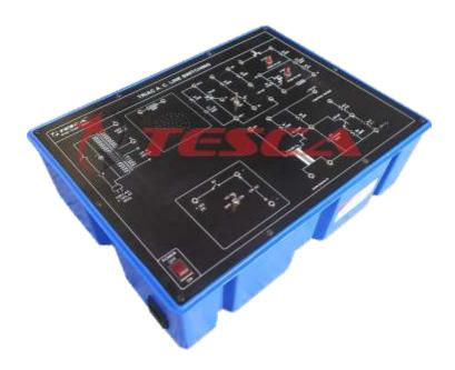
46524 Power Electronic Training Board has been designed specifically to study various switching techniques of TRIAC - a bidirectional silicon controlled switch. The phase control applications of TRIAC are included in another board 46521.
