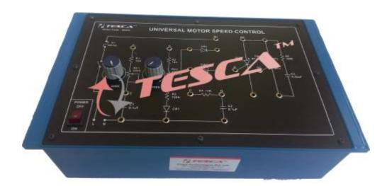
Power Electronic Training Board has been designed specifically for the study of speed control of universal motors in different modes, such universal motors are series wound motors capable of operating on both A.C. and D.C. supply. This Training Board is capable of controlling the speed of universal motor up to 1/4th H.P. Capacity.
